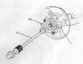
10) Remove sensor rotor (1) from wheel hub (2) as shown in the figure (if equipped with ABS).
