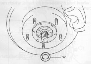
8) For 4WD vehicle, when installing circlip (1) to drive shaft, utilize screw hole in drive shaft to pull it out and bring large diameter (2) of circlip (1) at right as shown in the figure.
