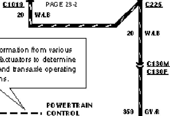
Uses information from various sensors & actuators to determine engine and transaxle operating conditions.
